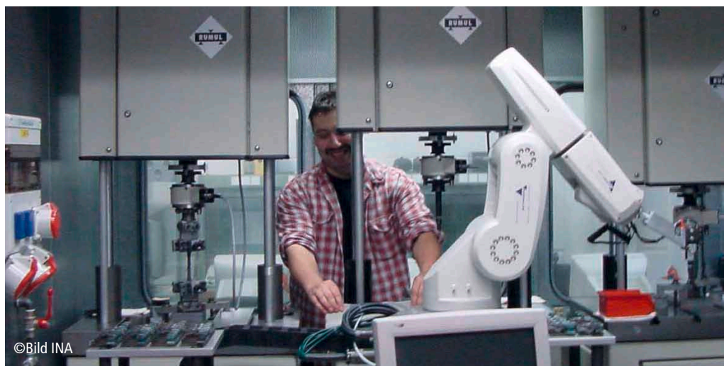
Automatic fatigue tests on rocker arm with manipulator
