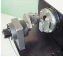
Gripping head for sheet metal tests
