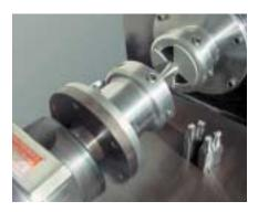
**Torsion tests** mounted gripping head for torsion tests
