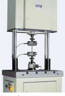
Resonant Testing Machine MIKROTRON 5/20 kN
