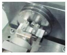
Bending tests on metal sheet
