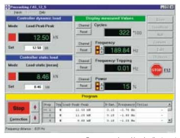
Frequency drop / load adjustment
